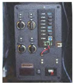
Image 1 - The upper left side of the Kendrick Model 208-IPP-C-3.0 Imaging Power Panel contains four 12-volt automobile-type outlets (two 5-amp, one 7-amp and one 10-amp). Other voltages are available by special order. The right side contains eight USB-3.0 ports (seven powered ports, plus one USB Standard B port). The bottom of the panel contains an LCD readout, an on/off switch and an Anderson-type jack for external power.
