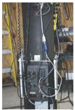
Image 3 - The Kendrick Model 208-IPP-C-3.0 Imaging Power Panel is shown installed on the main pier of the author's observatory. Two CCD cameras and a USB-to-serial adapter (for controlling the telescope mount) are plugged into the USB ports, while the 12-volt power plugs power two CCD cameras and telescope fans.
