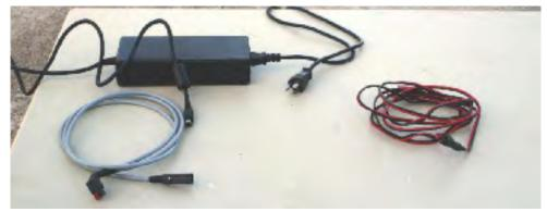
Image 2 - The IPP package ordered by the authored also included a 15-amp AC-to-12-volt DC power supply, a mini-DIN-to-Anderson plug (gray) cable and an Anderson plug-to-battery-terminal ring cable (red and black).
